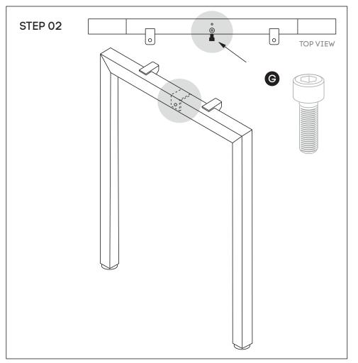
Using Allen Key provided, attach M8x20MM Socket head (G)-screw socket half way into leg for both legs (B)
