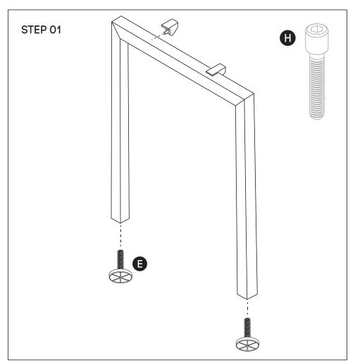
Using Allen Key provided, attach 2 plastic brackets per leg **(D)** (as per picture above) using M6x20MM **(H)** Socket head screw. Screw the feets **(E)** to the bottom of each leg **(B)**
