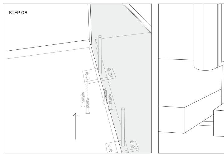
Second person to drill 4 holes into the brackets holes with provided wood screws into the underneath desktop. Please check the position of the rod brackets and bracket holes again before drilling the screws all the way through. Please tighten all the wood screws.
