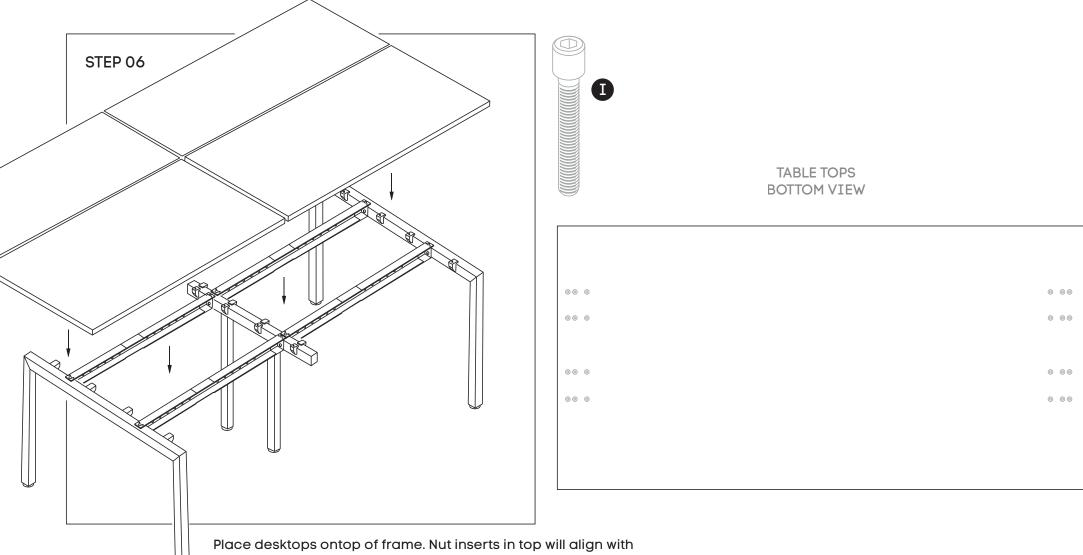
Place desktops ontop of frame. Nut inserts in top will align with plastic joiner brackets using M6x30MM (I) sockets attach tops to frame.
