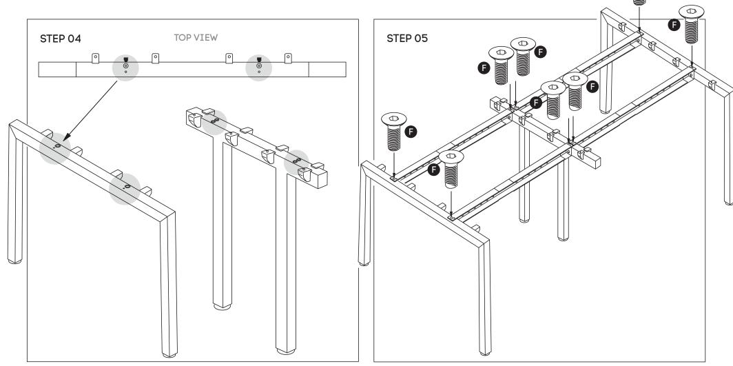
Attach beam **(D)** to legs **(B)** and Connector frame **(C)** using nut insert in legs. See point attached
