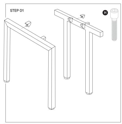
Using Allen Key provided, attach 2 plastic brackets per leg **(E)** (as per picture above) using M6x20MM **(H)** Socket head screw. Do the same with Connector frame **(C)**.
