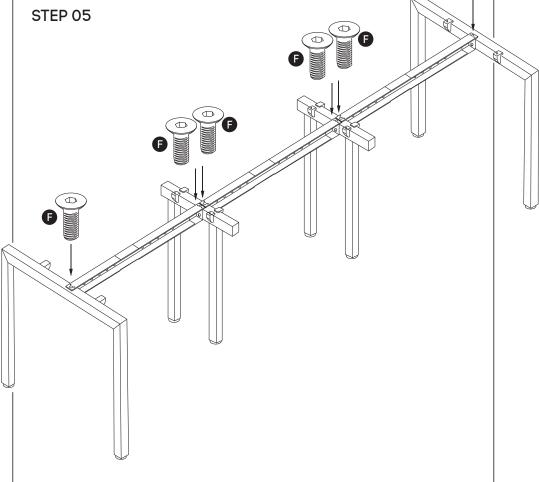
Attach beam **(D)** to legs **(B)** and Connector frame **(C)** using nut insert in legs. See point attached
