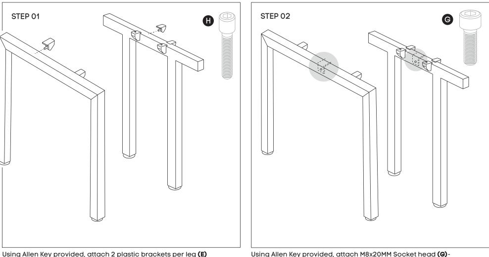
Using Allen Key provided, attach 2 plastic brackets per leg (E) (as per picture above) using M6x20MM (H) Socket head screw. Do the same with Connector frame (C). Using Allen Key provided, attach M8x20MM Socket head **(G)**screw socket half way into leg for both legs **(B)** and into Connector frame **(C)**.
