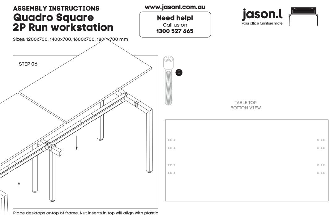
joiner brackets using M6x30MM (I) sockets attach tops to frame.
