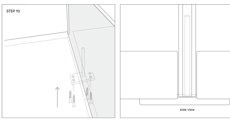
Second person to drill 4 holes into the brackets holes with provided wood screws into the underneath desktop. Please check the position of the rod brackets and bracket holes again before drilling the screws all the way through. Please tighten all the wood screws.
