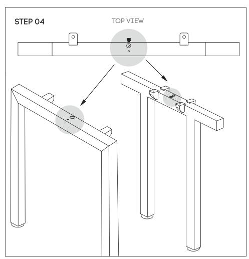
Attach beam **(F)** to legs **(C)** and Connector frame **(E)** using nut insert in legs. See point attached
