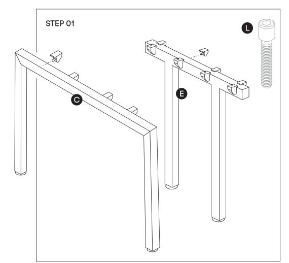
Using Allen Key provided, attach 4 plastic brackets **(H)** per leg **(C)** (as per picture above) using M6x20MM **(L)** Socket head screw. Do the same with Connector frame **(E)**.
