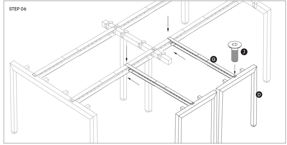
Attach the return beams **(G)** to return legs **(D)** using nut insert in legs. See point attached. Then, connect the hook of the return beam to the beam of the main structure. Repeat this step until the entire frame is complete.
