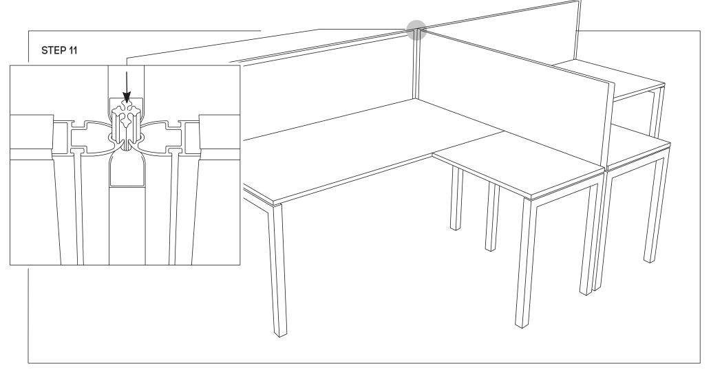
• Using an Allen key remove top 4 caps from all screens uprights. Bring four partition towards one another and slide the 4 way connector rod - down between the four screen uprights.
