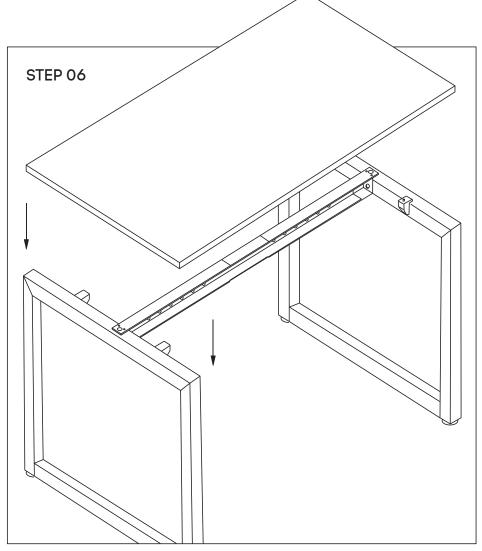
Place desktop on top of frame. Wood Screws to be drilled into the underneath Top.
