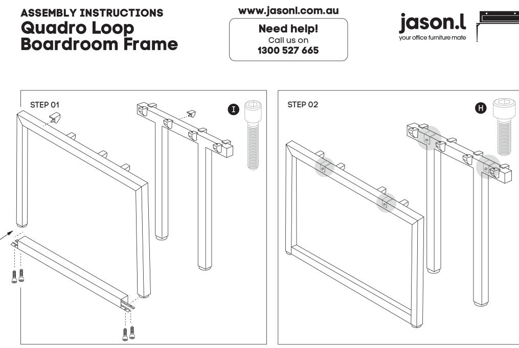
Using Allen Key provided, attach 4 plastic brackets per leg **(F)** (as per picture above) using M6x20MM **(I)** Socket head screw. Do the same with Connector frame **(D)**. Connect Loop Legs **(C)** to Bottom of Quadro Legs **(B)** by using 4 bolts per leg. Using Allen Key provided, attach M8x20MM Socket head **(H)**screw socket half way into leg for both legs **(B)** and into Connector frame **(D)**.
