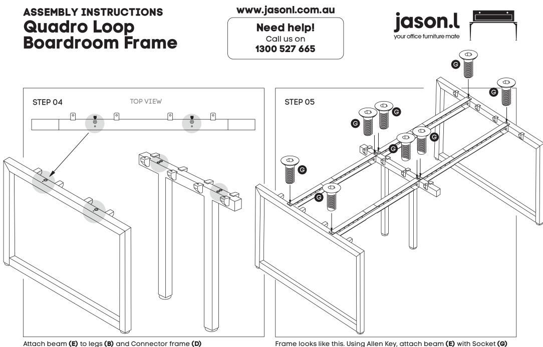
Attach beam **(E)** to legs **(B)** and Connector frame **(D)** using nut insert in legs. See point attached
