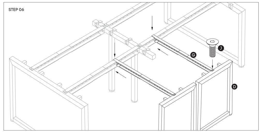
Attach the return beams **(G)** to return legs **(D)** using nut insert in legs. See point attached. Then, connect the hook of the return beam to the beam of the main structure. Repeat this step until the entire frame is complete.
