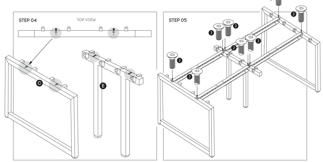
Attach main desk beams **(F)** to legs **(C)** and Connector frame **(E)** using nut insert in legs. See point attached
