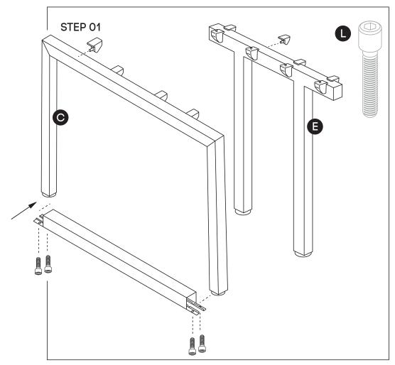
Using Allen Key provided, attach 4 plastic brackets (H) per leg (C) (as per picture above) using M6x20MM (L) Socket head screw. Do the same with Connector frame (E). Connect Loop Legs to Bottom of Quadro Legs (C) by using 4 bolts per leg.
