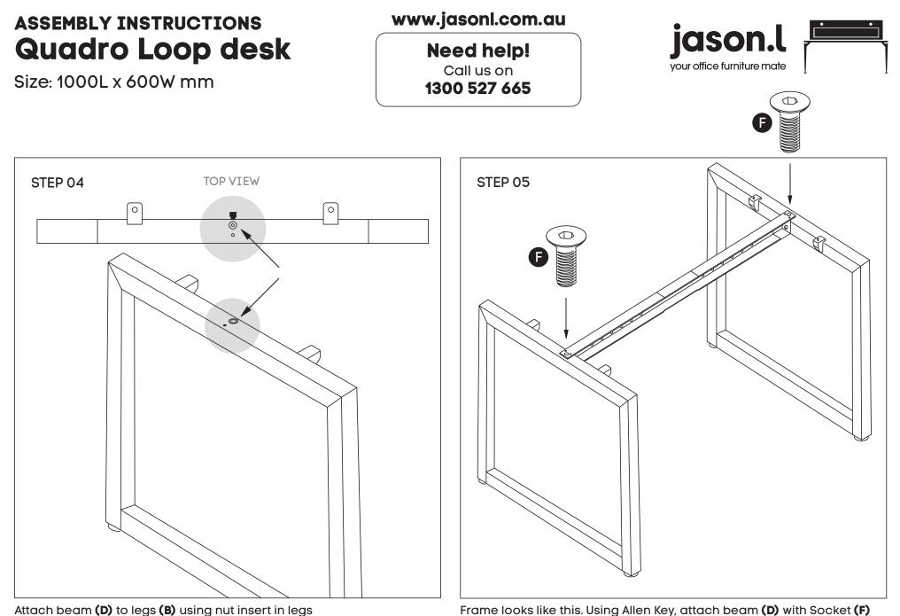
Attach beam **(D)** to legs **(B)** using nut insert in legs See point attached
