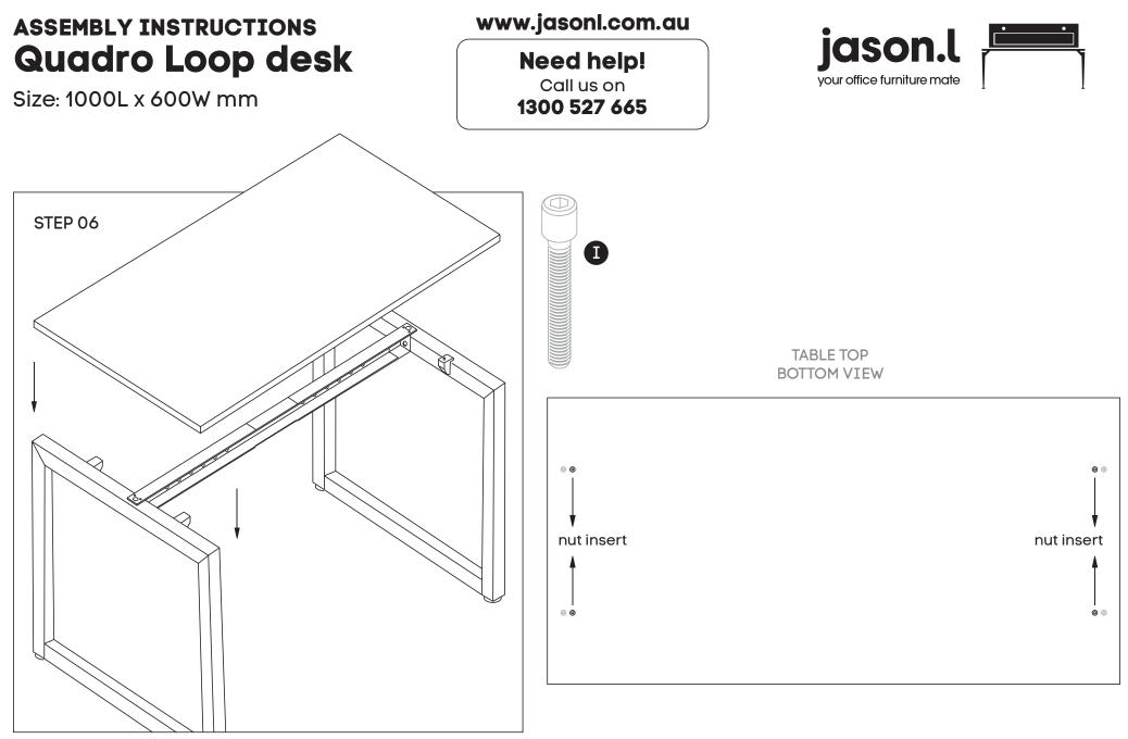
Place desktop ontop of frame. Nut inserts in top will align with plastic joiner brackets using M6x30MM **(I)** sockets attached top to frame.
