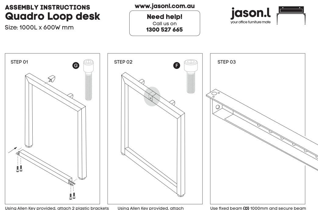
Using Allen Key provided, attach 2 plastic brackets per leg (E) (as per picture above) using M6x20MM (H) Socket head screw. Connect Loop Legs (C) to Bottom of Quadro Legs (B) by using 4 bolts per leg. Using Allen Key provided, attach M8x20MM Socket head **(G)**- screw socket half way into leg for both legs **(B)**
