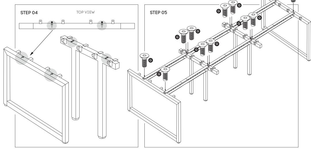
Attach beam **(E)** to legs **(B)** and Connector frame **(D)** using nut insert in legs. See point attached
