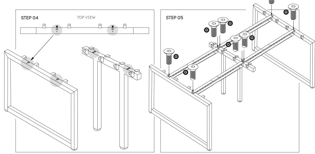
Attach beam **(E)** to legs **(B)** and Connector frame **(D)** using nut insert in legs. See point attached
