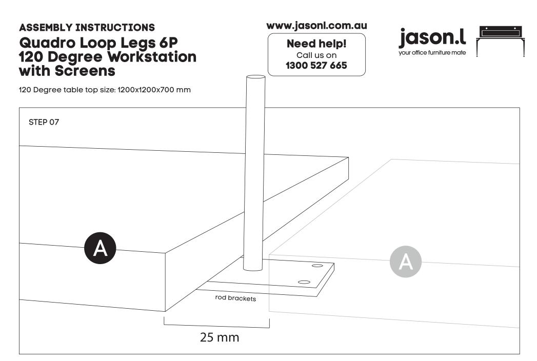
Drop the desk mounted screen in between the two tops (A). Now please insert 2 rod brackets that will hold each screen to the desks on either side.
