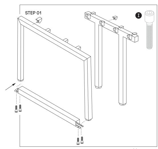
Using Allen Key provided, attach 4 plastic brackets per leg **(F)** (as per picture above) using M6x20MM **(I)** Socket head screw. Do the same with Connector frame **(D)**. Connect Loop Legs **(C)** to Bottom of Quadro Legs **(B)** by using 4 bolts per leg
