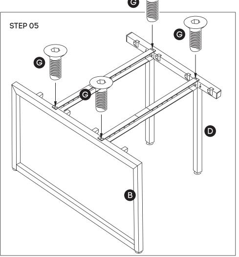
Frame looks like this. Using Allen Key, attach beam (E) with Socket (G)
