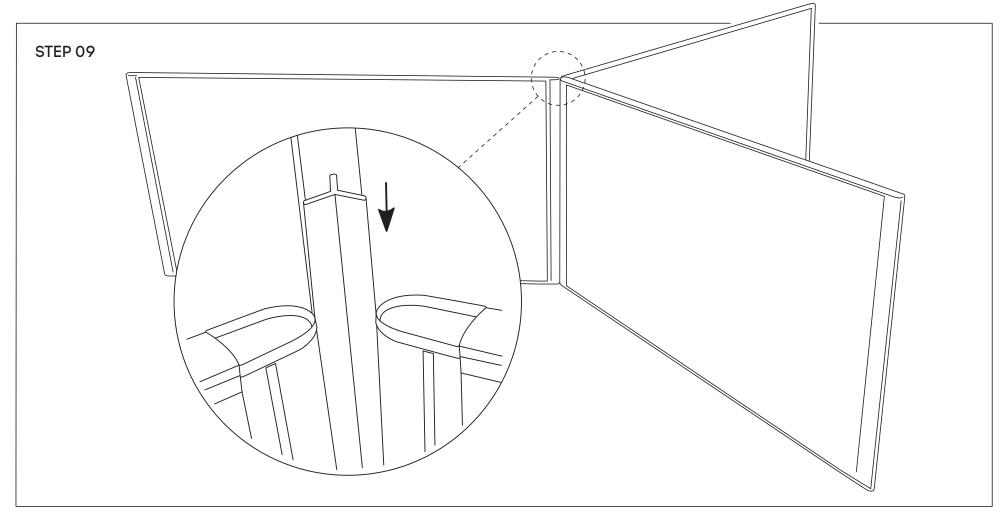
Using an allen key, please remove 3 caps from all screens. Bring 3 partitions towards one another and slide the 3-way 120 degree connector -down between the three screen uprights.
