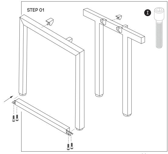
Using Allen Key provided, attach 2 plastic brackets per leg **(F)** (as per picture above) using M6x20MM **(I)** Socket head screw. Do the same with Connector frame **(D)**. Connect Loop Legs **(C)** to Bottom of Quadro Legs **(B)** by using 4 bolts per leg
