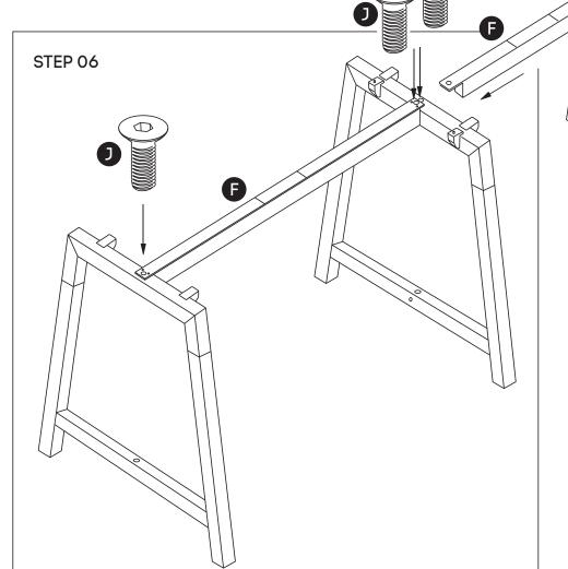
Frame looks like this. Using Allen Key, attach Upper Beams **(F)** with Sockets **(J)**.
