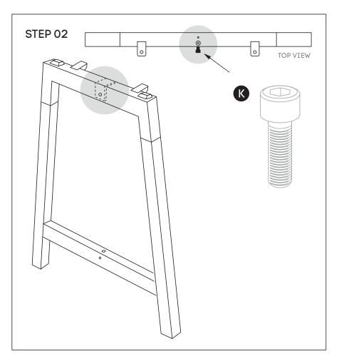
Using Allen Key provided, attach M8x20MM Socket head **(K)**-screw socket half way into legs.
