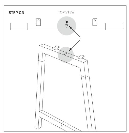
Attach Upper Beams **(F)** to legs using nut insert. See point attached
