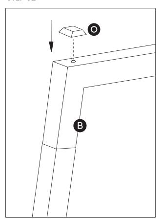
Now use corner pads **(O)** to cover the holes where just inserted the head screw sockets.
