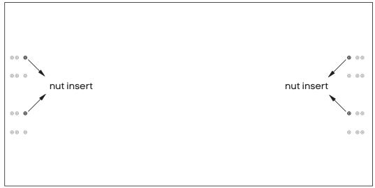
Place desktops (A) ontop of frames. Nut inserts in top will align with plastic joiner brackets using M6x30MM (K) sockets attached tops to frames.
