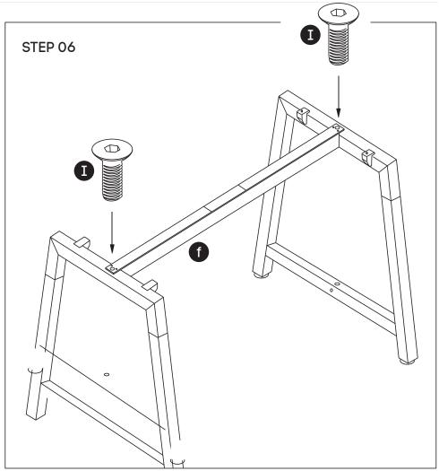
Frame looks like this. Using Allen Key, attach Upper Beam **(f)** with Sockets **(I)**.
