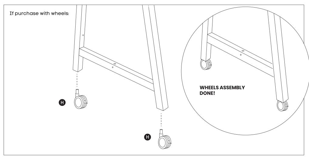
Replace Feet on the bottom of each leg with wheels (H)
