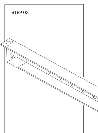
Use fixed beam **(E)** and secure beam using screws provided to suit desk
