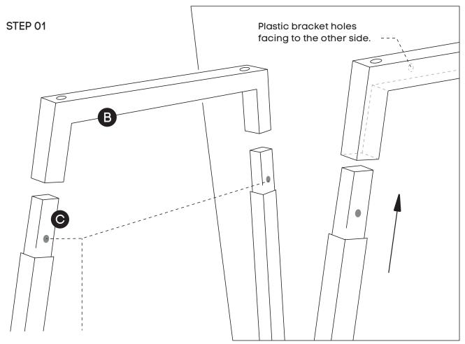
Both legs must have the colour sticker facing away from where the plastic brackets are inserted.
