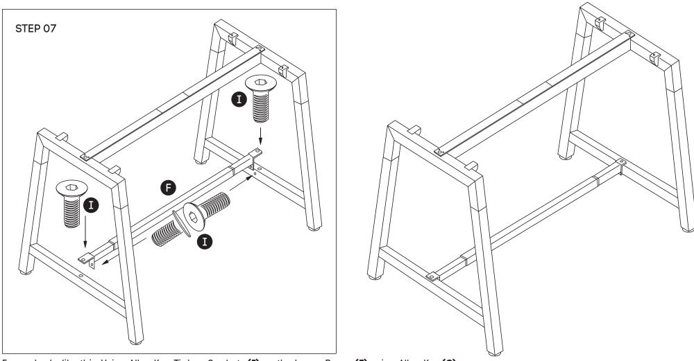
Frame looks like this. Using Allen Key. Tighen Sockets (I) on the Lower Beam (F) using Allen Key (O). Insert plastic spacers to improve regidity. Attach two Sockets (I) to the side of the lower side beams (as shown in the picture).
