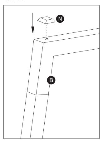
Now use corner pads (N) to cover the holes where just inserted the head screw sockets.
