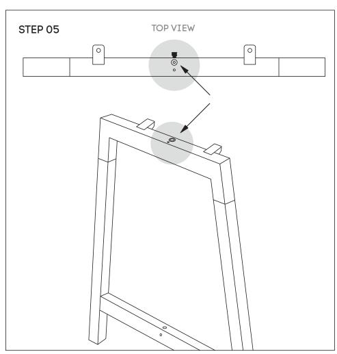
Attach Upper Beam **(F)** to legs using nut insert. See point attached
