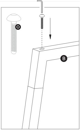
Insert the Leg wood add on **(C)** into the Leg Quadro A (Half leg) **(B)**. Using Allen Key provided, attach mushroom head screw **(O)** for all legs.
