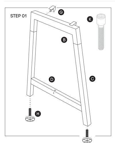
Using Allen Key provided, attach 2 plastic brackets per leg (G) (as per picture above) using M6x20MM (K) Socket head screw. Screw the feets (H) to the bottom of each Leg wood add on (C).
