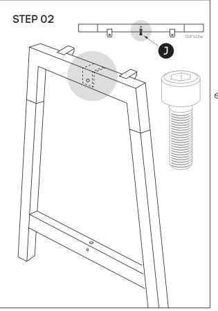
Using Allen Key provided, attach M8x20MM Socket head (1) - screw socket half way into leg for both legs
