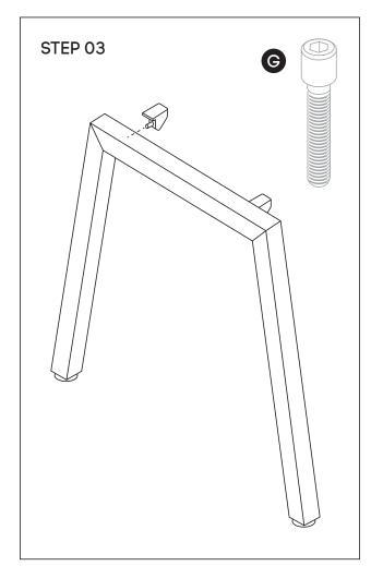
Using Allen Key provided, attach 2 plastic brackets per leg **(D)** (as per picture above) using M6x20MM **(G)** Socket head screw
