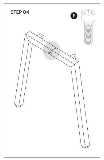
Using Allen Key provided, attach M8x20MM Socket head **(F)**- screw socket half way into leg for both legs **(B)**
