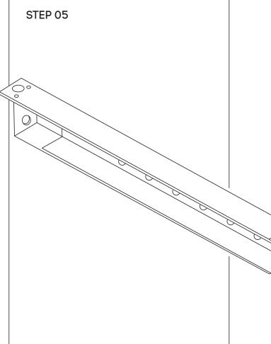
Use fixed beam **(C)** 1000mm and secure beam using screws provided to suit 1000mm desk
