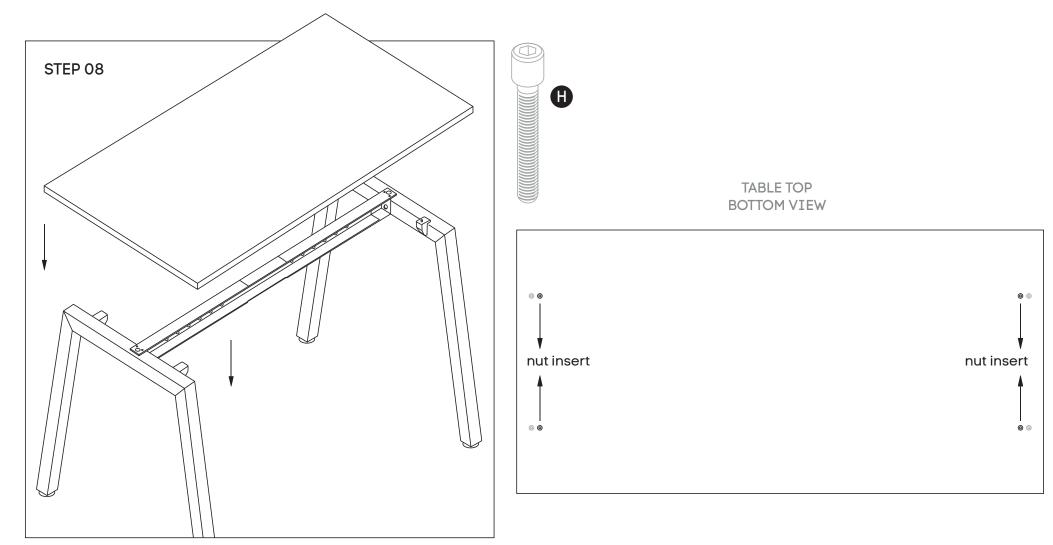
Place desktop ontop of frame. Nut inserts in top will align with plastic joiner brackets using M6x30MM **(H)** sockets attached top to frame.
