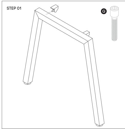
Using Allen Key provided, attach 2 plastic brackets per leg (D)
