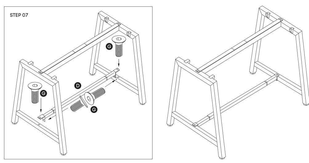
Frame looks like this. Using Allen Key. Tighen Sockets (G) on the Lower Beam (D) using Allen Key (J). Insert plastic spacers to improve regidity. Attach two Sockets (G) to the side of the lower side beams (as shown in the picture).
