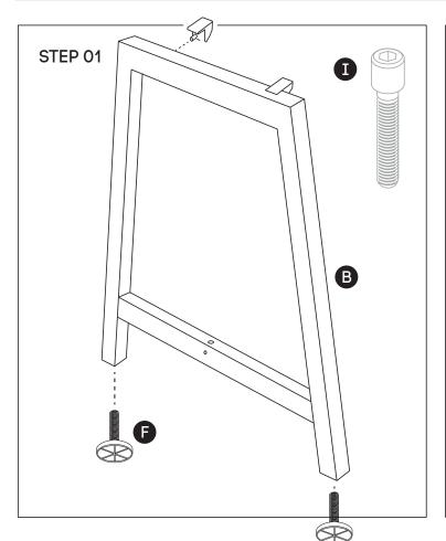
Using Allen Key provided, attach 2 plastic brackets per leg (**D**) (as per picture above) using M6x20MM (**I**) Socket head screw. Screw the feets (**F**) to the bottom of each leg (**B**)
