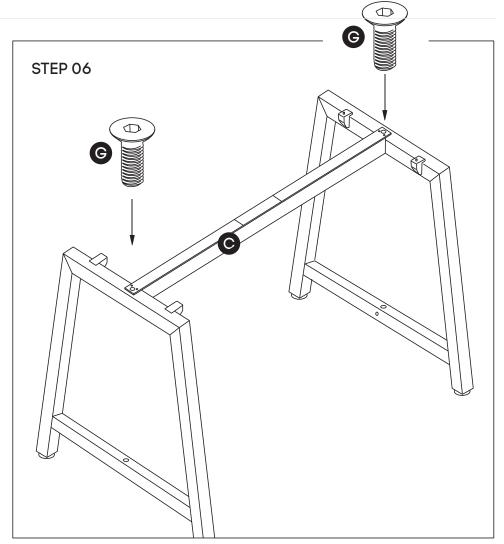
Frame looks like this. Using Allen Key, attach Upper Beam **(C)** with Sockets **(G)**.
