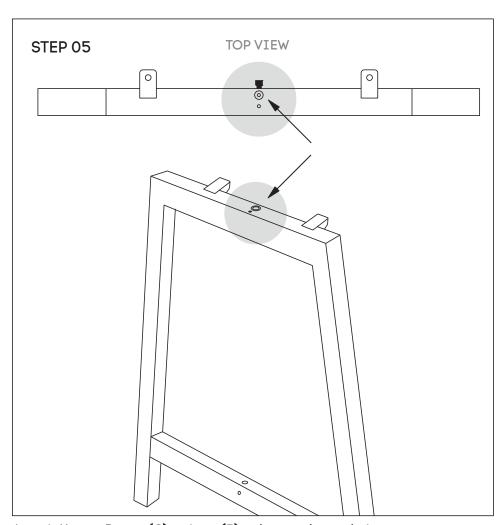
Attach Upper Beam **(C)** to legs **(B)** using nut insert in legs. See point attached
