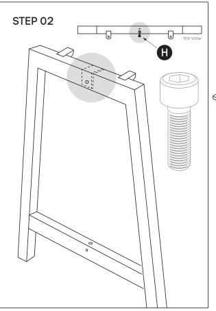
Using Allen Key provided, attach M8x20MM Socket head (H)- screw socket half way into leg for both legs (B)
