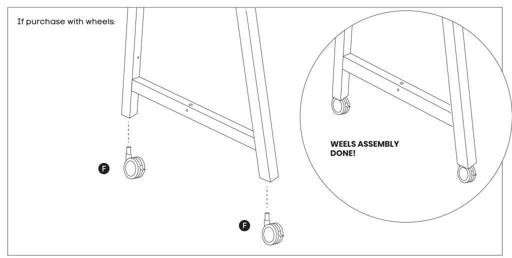
Replace Feet on the bottom of each leg with wheels (Fa)
