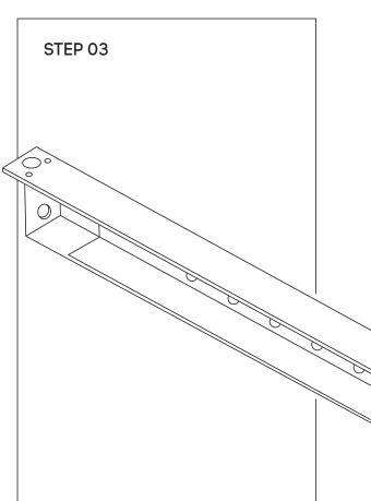
Use fixed beam **(C)** and secure beam using screws provided to suit desk
