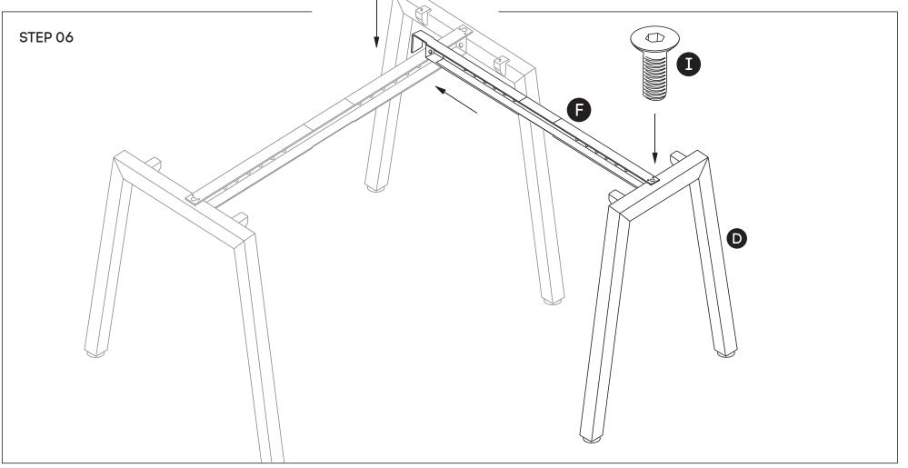
Now attach the return beam (F) to return leg (D) using nut insert in legs. See point attached. Then, connect the hook of the return beam to the beam of the main structure.
