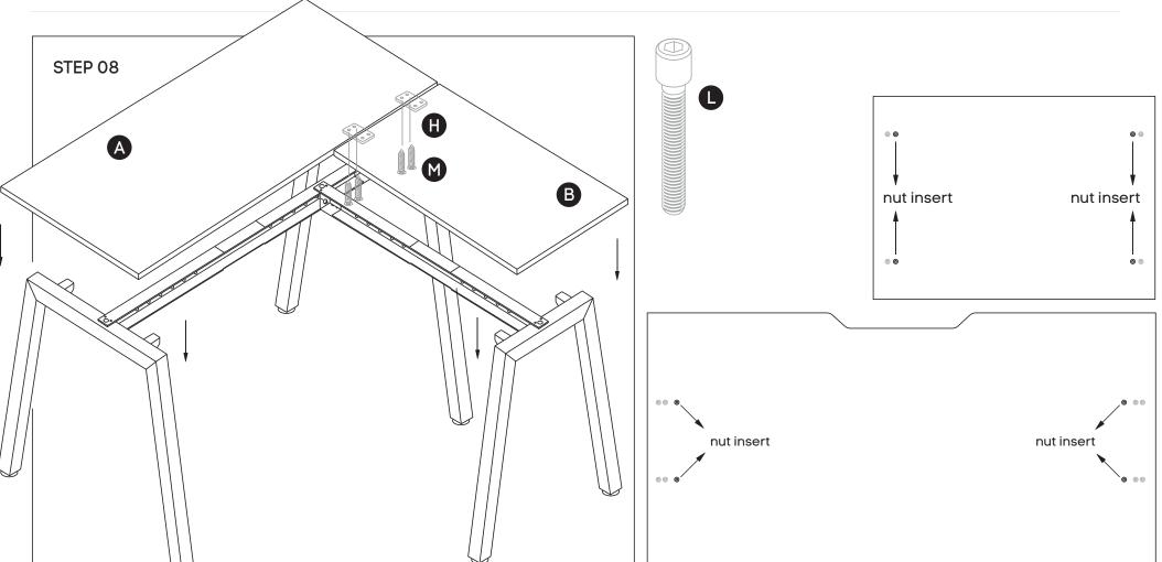
Place table top (A) ontop of frame - with cutout at the back of the desk. Using nut inserts in the desk, use M6x30mm socket (L) and attach desktop to the frame. Using nut inserts in the desktop, use M6x30mm socket (L) and attach desktop (B) to the frame. Once desktop are attached and secure to the frame, use woods screws and secure joiner plates to the underside of desktop A.
