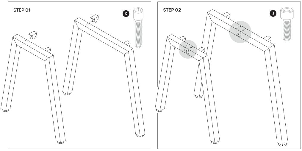
Using Allen Key provided, attach 2 plastic brackets (G) per legs (C & D) (as per picture above) using M6x20MM (K) Socket head screw Using Allen Key provided, attach M8x20MM Socket head (J)screw socket half way into leg for three legs (C & D)
