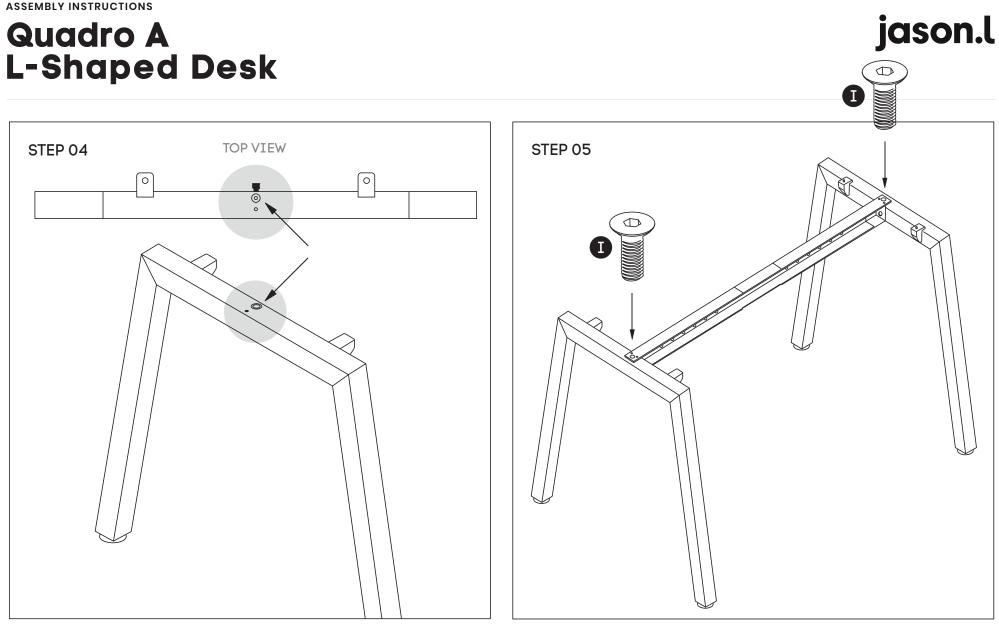
Attach beam **(E)** to legs **(C)** using nut insert in legs. See point attached Frame looks like this. Using Allen Key, attach beam (E) with Socket (I)
