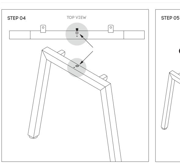
Attach beam **(C)** to legs **(B)** using nut insert in legs. See point attached Frame looks like this. Using Allen Key, attach beam (C) with Socket (E)
