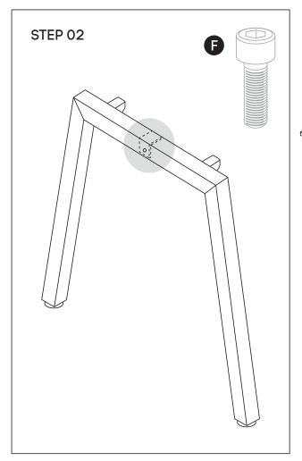
Using Allen Key provided, attach M8x20MM Socket head **(F)**- screw socket half way into leg for both legs **(B)**
