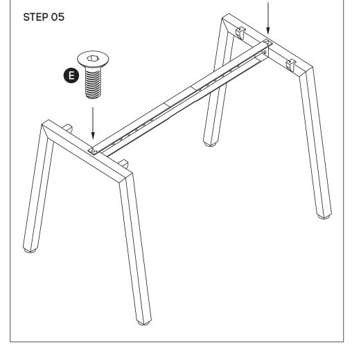
Attach beam **(C)** to legs **(B)** using nut insert in legs See point attached
