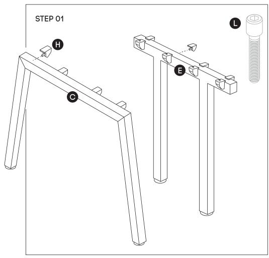
Using Allen Key provided, attach 4 plastic brackets (H) per leg (C) (as per picture above) using M6x20MM (L) Socket head screw. Do the same with Connector frame (E).
