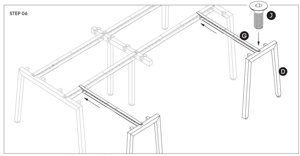
Now attach the return beams (G) to return legs (D) using nut insert in legs. See point attached.
