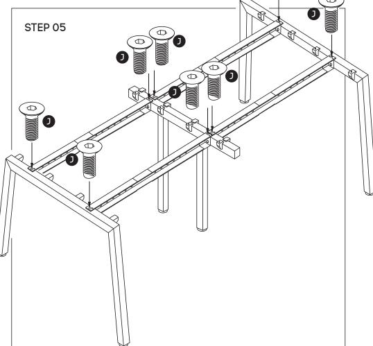
Attach beam **(F)** to legs **(C)** and Connector frame **(E)** using nut insert in legs. See point attached
