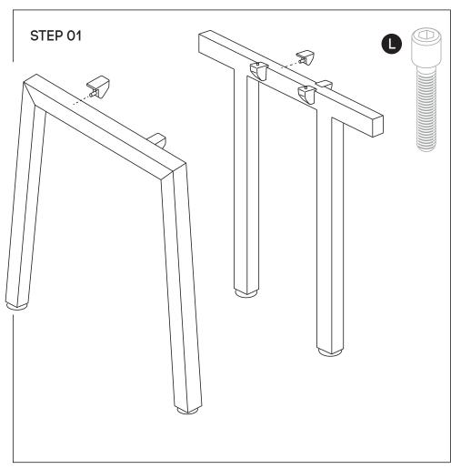
Using Allen Key provided, attach 2 plastic brackets per leg (C)(D) (as per picture above) using M6x20MM (L) Socket head screw. Do the same with Connector frame (E).
