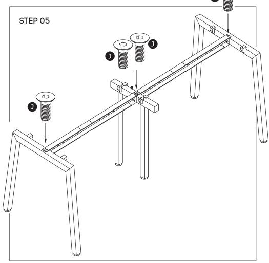
Attach beam **(F)** to legs **(C)** and Connector frame **(E)** using nut insert in legs. See point attached
