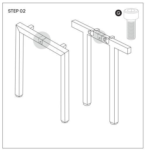
Using Allen Key provided, attach M8x20MM Socket head (G)-screw socket half way into leg for both legs (B) and into Connector frame (C).
