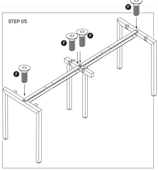
Frame looks like this. Using Allen Key, attach beam (D) with Socket (F)
