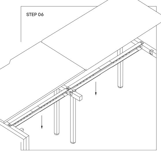
Place the desktop on top of the frame. Please place the legs ideally indented around 300mm from each end left and right of the Tops, Place the legs centred at the same distance equally from the front and back of the top.
