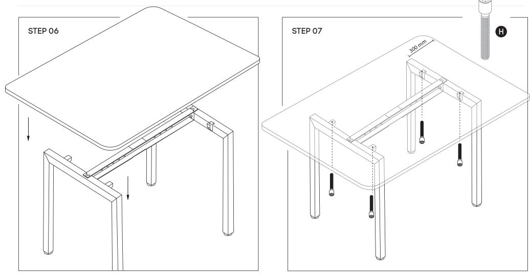
Place the desktop on top of the frame. Please place the legs ideally indented around 300mm from each end left and right of the Tops, Place the legs centred at the same distance equally from the front and back of the top.
