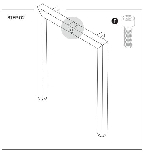
Using Allen Key provided, attach M8x20MM Socket head **(F)**-screw socket half way into leg for both legs **(B)**
