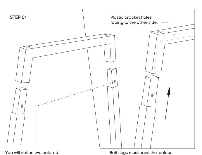
Insert the bottom of the legs as shown in the illustration. Using Allen Key provided, attach Mushroom Head Screw (N) - for all legs.
