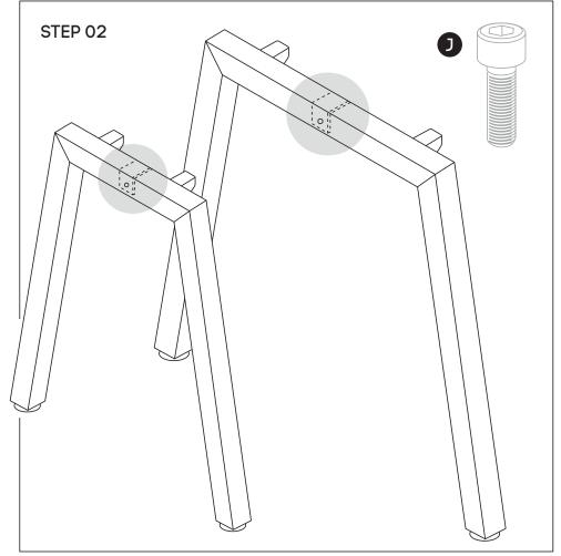
Using Allen Key provided, attach M8x20MM Socket head (J)-screw socket half way into leg for three legs (C & D)
