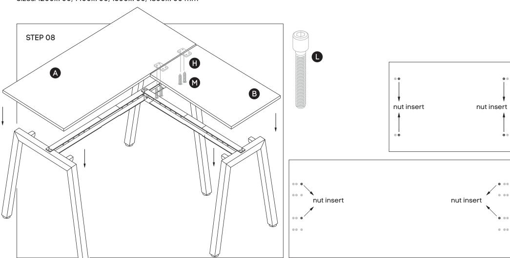
Place table top (A) ontop of frame. Using nut inserts in the desk, use M6x30mm socket (L) and attach desktop to the frame. Using nut inserts in the desktop, use M6x30mm socket (L) and attach desktop (B) to the frame. Once desktop are attached and secure to the frame, use woods screws and secure joiner plates to the underside of desktop A.
