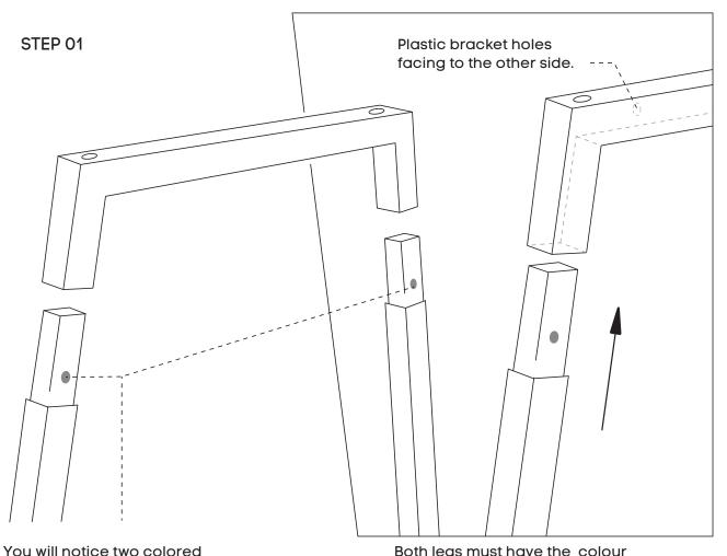
Both legs must have the colour sticker facing away from where the plastic brackets are inserted.
