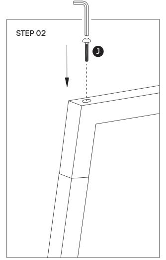
Insert the bottom of the legs as shown in the illustration. Using Allen Key provided, attach Mushroom Head Screw (J) - for all legs.
