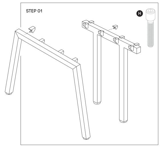
Using Allen Key provided, attach 4 plastic brackets per leg **(E)** (as per picture above) using M6x20MM **(H)** Socket head screw. Do the same with Connector frame **(C)**.
