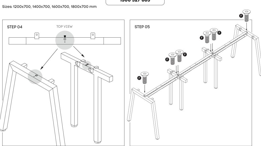
Attach beam **(D)** to legs **(B)** and Connector frame **(C)** using nut insert in legs. See point attached
