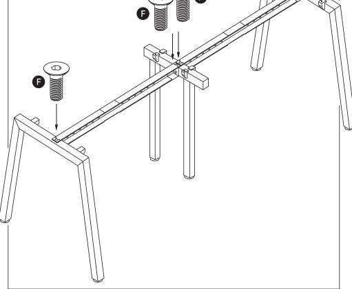
Attach beam **(D)** to legs **(B)** and Connector frame **(C)** using nut insert in legs. See point attached
