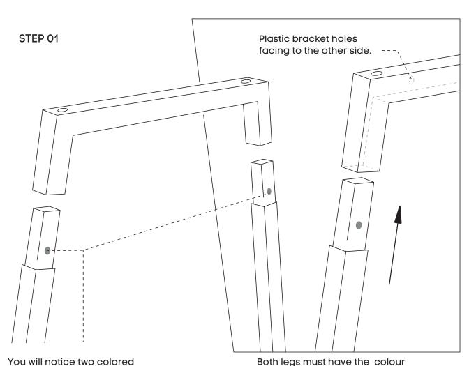
Insert the bottom of the legs as shown in the illustration. Using Allen Key provided, attach Mushroom Head Screw (I) - for all legs.
