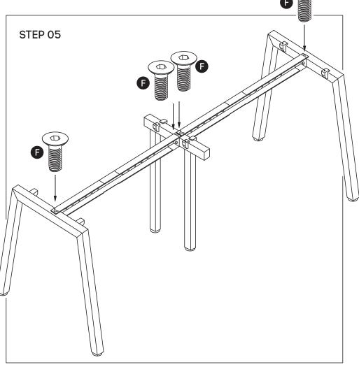
Frame looks like this. Using Allen Key, attach beam (D) with Socket (F)
