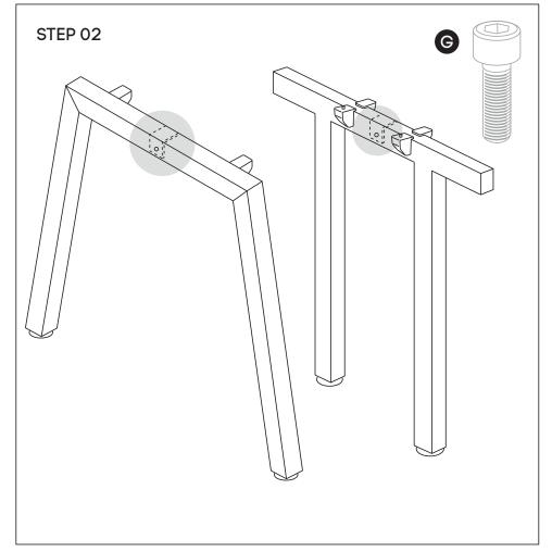
Using Allen Key provided, attach M8x20MM Socket head (G)-screw socket half way into leg for both legs (B) and into Connector frame (C).
