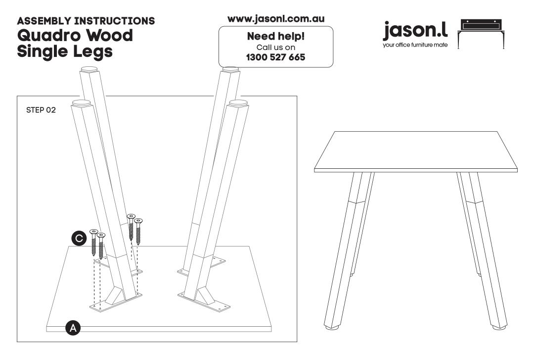
Ask a second person to help turn the table and base over. Screw the table tops to the bases using woodscrews (C) through the following holes.
