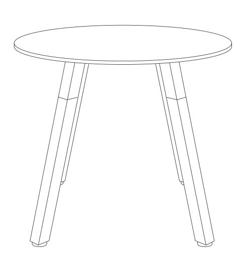
Ask a second person to help turn the table and base over. Screw the table tops to the bases using woodscrews (C) through the following holes.
