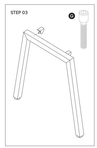
Using Allen Key provided, attach 2 plastic brackets per leg (D) (as per picture above) using M6x20MM (G) Socket head screw
