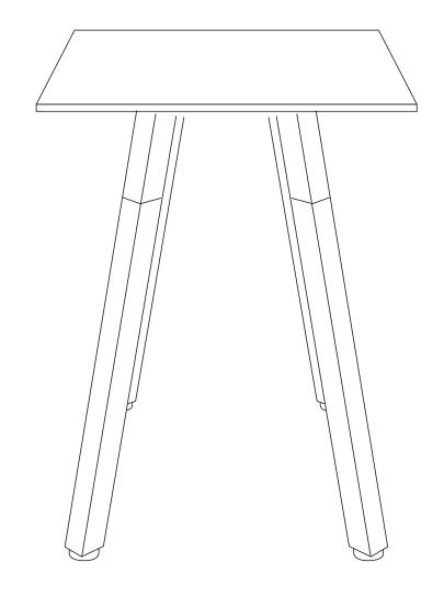
Ask a second person to help turn the table and base over. Screw the table tops to the bases using woodscrews (C) through the following holes.
