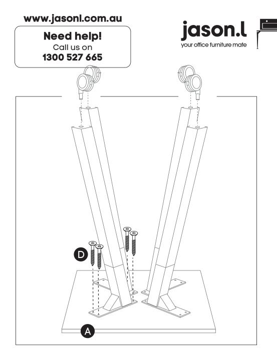
Ask a second person to help turn the table and base over. Screw the table tops to the bases using woodscrews **(D)** through the following holes. Screw the wheels to the bottom of each Leg.
