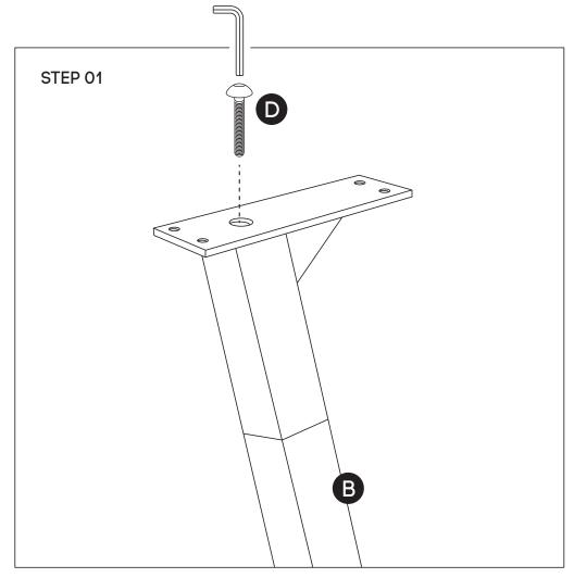
Using Allen Key provided, attach Mushroom Head Screw **(D)** for all legs as shown in the illustration.
