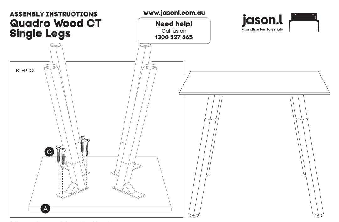
Ask a second person to help turn the table and base over. Screw the table tops to the bases using woodscrews (C) through the following holes.
