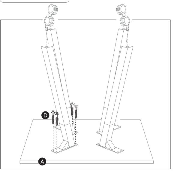
Ask a second person to help turn the table and base over. Screw the table tops to the bases using woodscrews **(D)** through the following holes. Screw the wheels to the bottom of each Leg.
