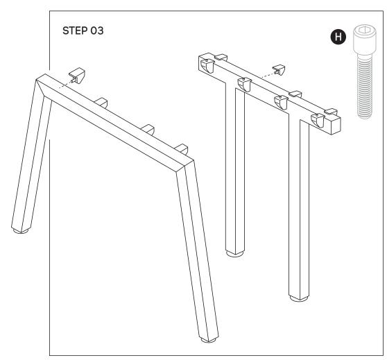
Using Allen Key provided, attach 4 plastic brackets per leg **(E)** (as per picture above) using M6x20MM **(H)** Socket head screw. Do the same with Connector frame **(C)**.
