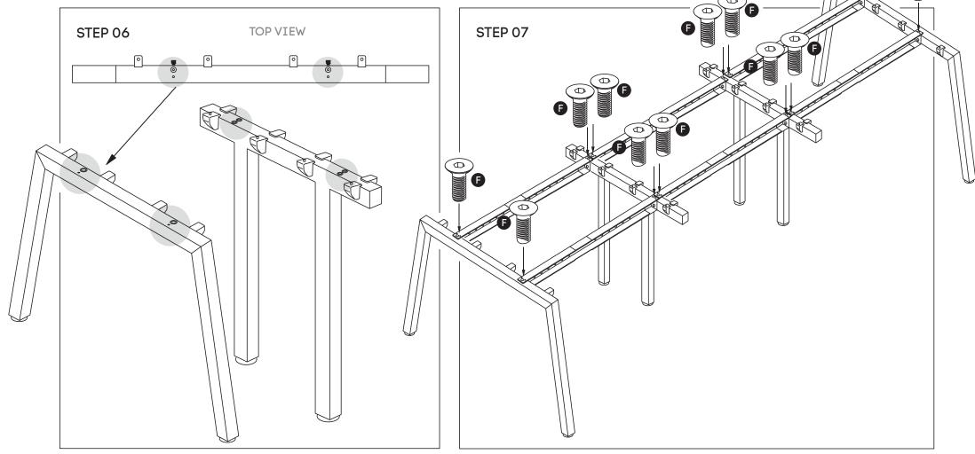
Attach beam **(D)** to legs **(B)** and Connector frame **(C)** using nut insert in legs. See point attached
