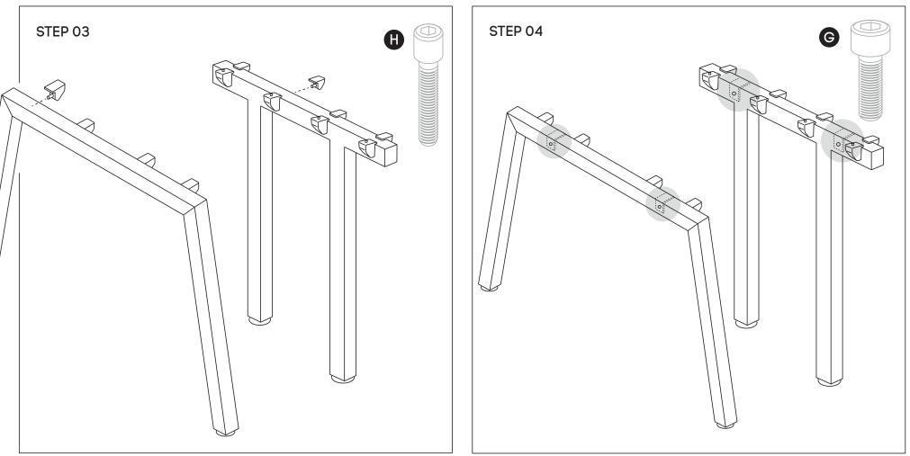
Using Allen Key provided, attach 4 plastic brackets per leg **(E)** (as per picture above) using M6x20MM **(H)** Socket head screw. Do the same with Connector frame **(C)**.
