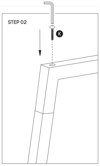
Insert the bottom of the legs as shown in the illustration. Using Allen Key provided, attach Mushroom Head Screw (K) - for all legs.
