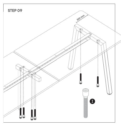
Please tighten M6x30MM Socket head (I) through the plastic brackets into the underneath of the tops.
