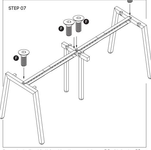
Attach beam **(D)** to legs **(B)** and Connector frame **(C)** using nut insert in legs. See point attached
