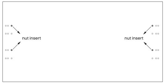
Place desktop ontop of frame. Nut inserts in top will align with plastic joiner brackets using M6x30MM (J) sockets attached top to frame.
