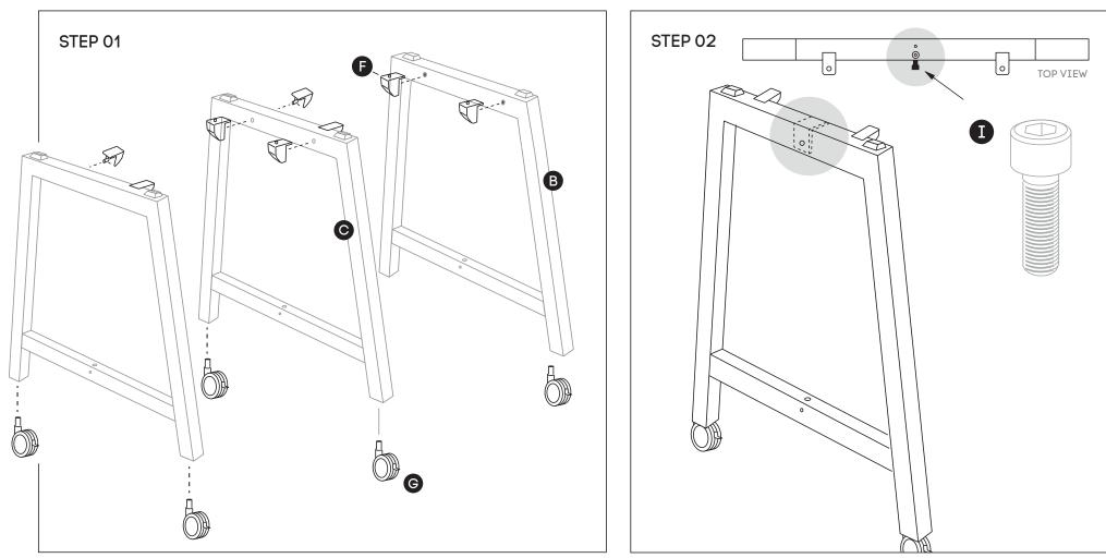
Using Allen Key provided, attach 2 plastic brackets (F) per exterior leg (B) (as per picture above) using M6x20MM (J) Socket head screw. Attach 4 plastic brackets (F) to the Intermediate leg (C) using M6x20MM (J). Screw the wheels (G) to the bottom of each Leg. Using Allen Key provided, attach M8x20MM Socket head **(I)**-screw socket half way into legs.
