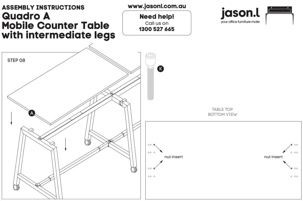
Place desktops **(A)** ontop of frames. Nut inserts in top will align with plastic joiner brackets using M6x30MM **(K)** sockets attached tops to frames.
