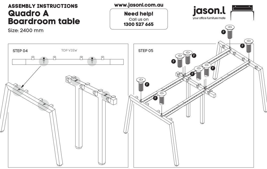
Attach beam **(D)** to legs **(B)** and Connector frame **(C)** using nut insert in legs. See point attached
