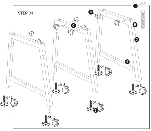
Using Allen Key provided, attach 2 plastic brackets (H) per exterior leg (as per picture above) using M6x20MM (L) Socket head screw. Attach 4 plastic brackets (H) to the Intermediate leg (C) using M6x20MM (L). Screw the feets or wheels (if you purchase with wheels option) (I) to the bottom of each Leg wood add on (D).
