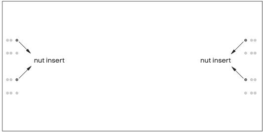
Place desktops (A) ontop of frames. Nut inserts in top will align with plastic joiner brackets using M6x30MM (M) sockets attached tops to frames.
