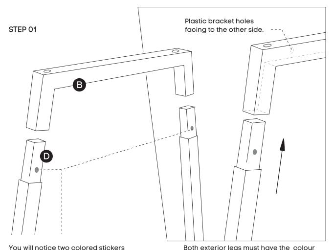
Insert the Leg wood add on **(D)** into the Leg Quadro A (Half leg) **(B)** and also intermediate leg **(C)**. Using Allen Key provided, attach mushroom head screws **(P)** for all legs.
