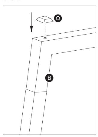
Now use corner pads (O) to cover the holes where just inserted the head screw sockets.
