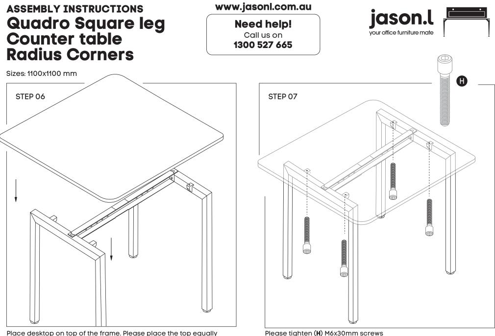
Place desktop on top of the frame. Please place the top equally centred at the same distance from left and right of the leg frame and then please tighten screws using M6x30MM (**H**) into the underneath of the tops.
