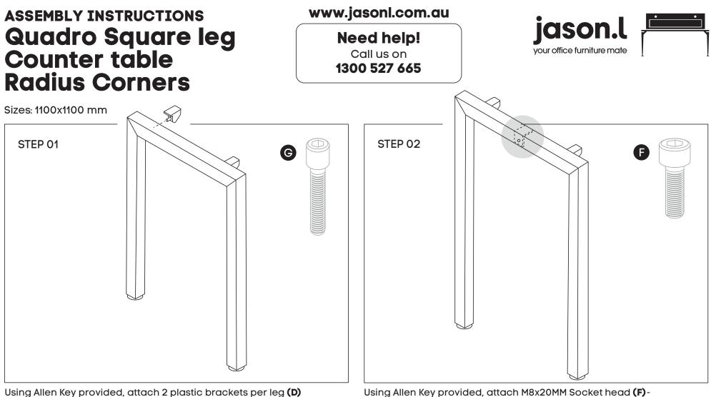
(as per picture above) using M6x20MM (G) Socket head screw
