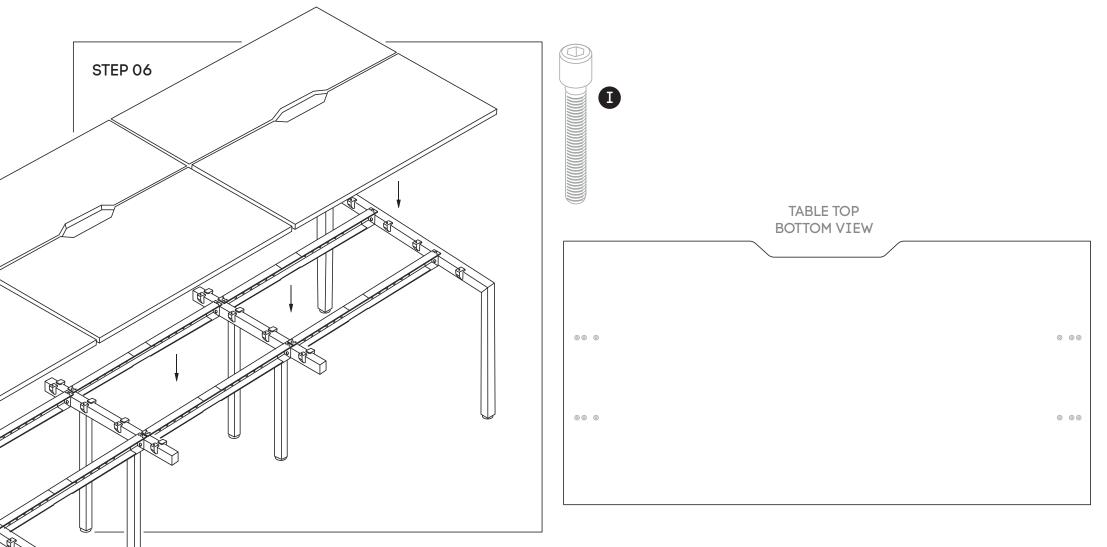
Place desktops ontop of frame - with cutout at the back of the desk. Nut inserts in top will align with plastic joiner brackets using M6x30MM (I) sockets attached tops to frame.
