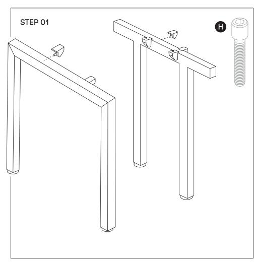
Using Allen Key provided, attach 2 plastic brackets per leg **(E)** (as per picture above) using M6x20MM **(H)** Socket head screw. Do the same with Connector frame **(C)**.
