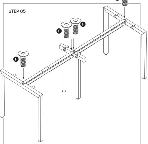
Attach beam **(D)** to legs **(B)** and Connector frame **(C)** using nut insert in legs. See point attached
